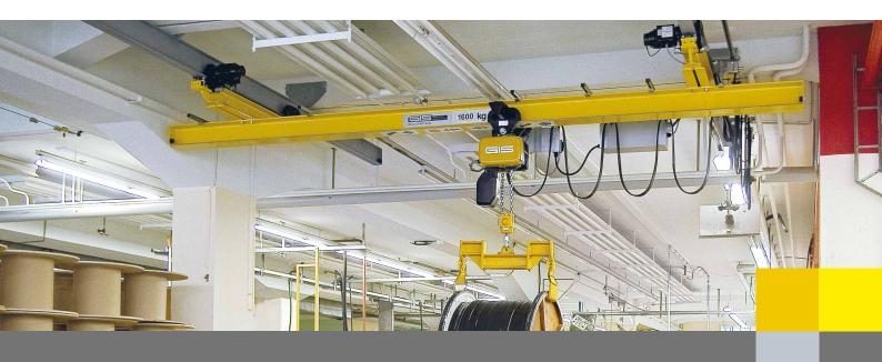
GIS travelling cranes define the overhead material transport up to 5000 kg lifting capacity in terms of efficiency. Our objective is rational and area covering goods handling. Based on structural and customer's requirements, we offer and realise the appropriate, robust and durable solution in design, ergonomics and safety.
